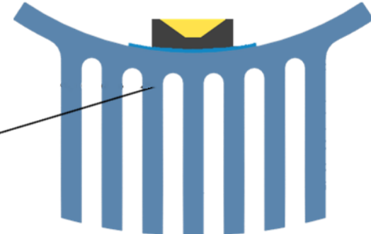
new: Alu-compound heat sink = case PlastFormance
